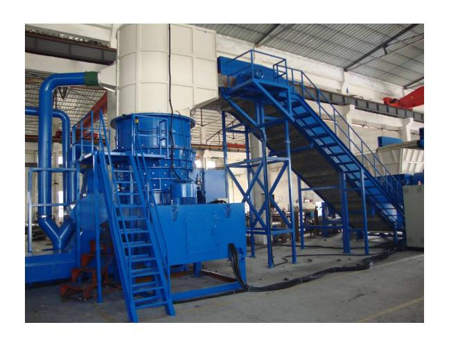
THIS PICTURE ABOVE SHOWS OUR VERTICAL GRINDER DENSIFIER FOR SCRAP PROCESSING APPLICATIONS....
