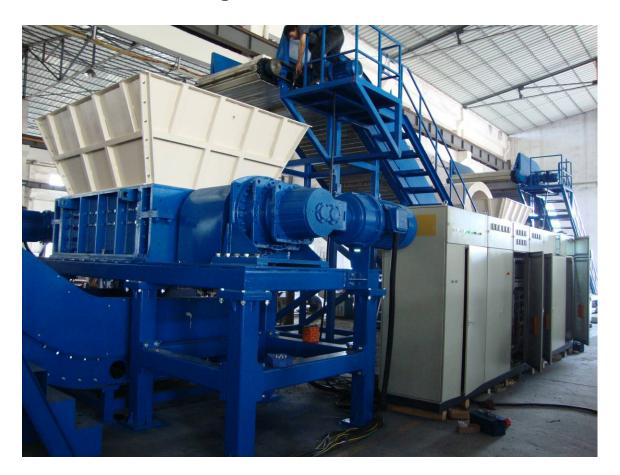
The Tertiary Shredder ( 3<sup>rd</sup> in Line ) in this data is either a Model 7272 shredder or a Model 5444 shredder to shred material from the Secondary Shredder into a rought 2" cut.
