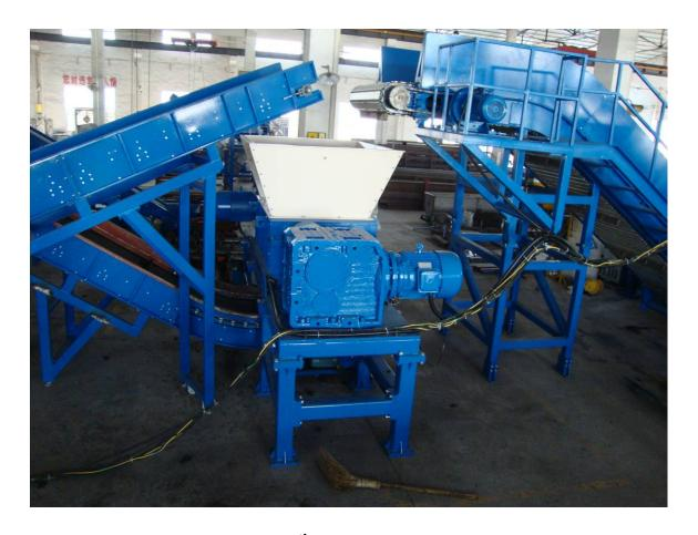
The Fourth Shredder ( 4<sup>th</sup> in Line ) in this data is either a Model 7272 shredder or a Model 5444 shredder to shred material from the Tertiary shredder into a more uniform 2" size.
