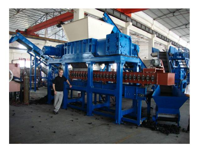
If the system needs to produce a smaller 1" particle then the system will use two or three more shredders to accomplish the progressive grinding to this particle size.
