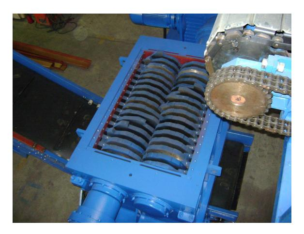
The Sixth shredder (6<sup>th</sup> in Line) can be either a Model 7272 shredder or a Model 5444 shredder with a 1" cut.
