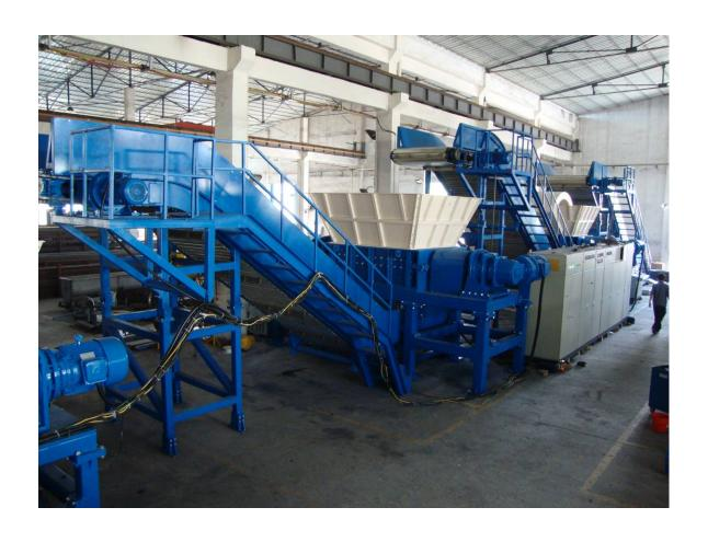
THIS PICTURE ABOVE SHOWS ONE OF OUR FOUR SHREDDER PROCESSING SYSTEMS WITH TWO 7272 SHREDDERS AND TWO 5444 SHREDDERS IN A LINEAR FORM.
