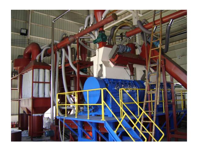
THIS PICTURE ABOVE SHOWS A DUAL GRANULAR SYSTEM WITH ITS ASSOCIATED SCREENING SYSTEM AND AIR SYSTEM AND MAGNETIC SYSTEM...
