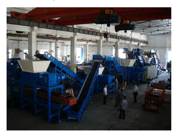
The Primary Shredder in this data is a Model 7272 Shredder to pre shred material into a rough 6" cut.
