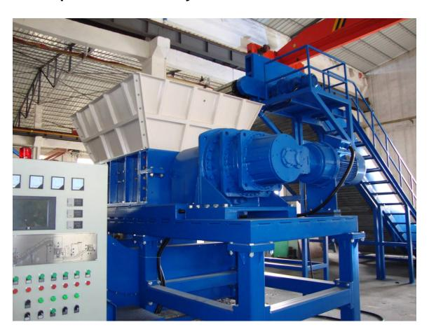
The picture above shows a system designed to process a wide range of materials in this case, 500 to 600 Truck, and Passenger tires, per hour, into a 2" fuel chip or shred size.
