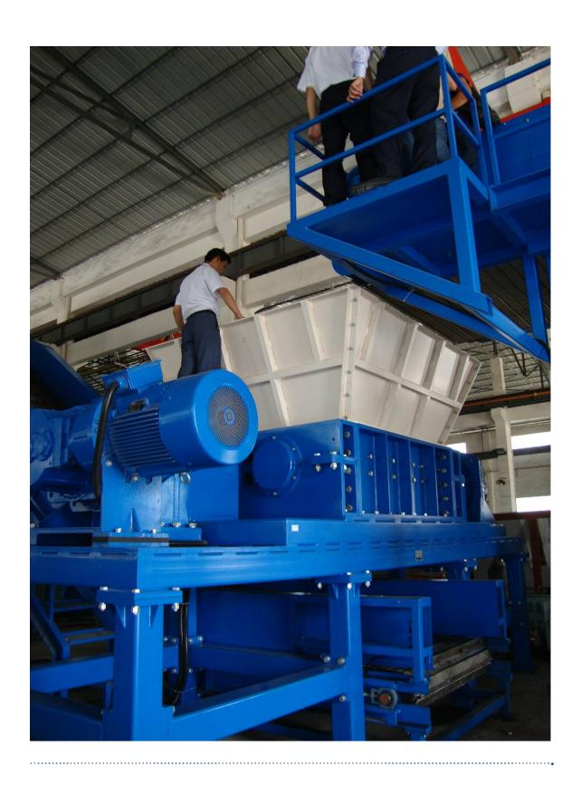
The Secondary Shredder in this data is another Model 7272 shredder used to shred material from the Primary Shredder into a rough 3" cut.
