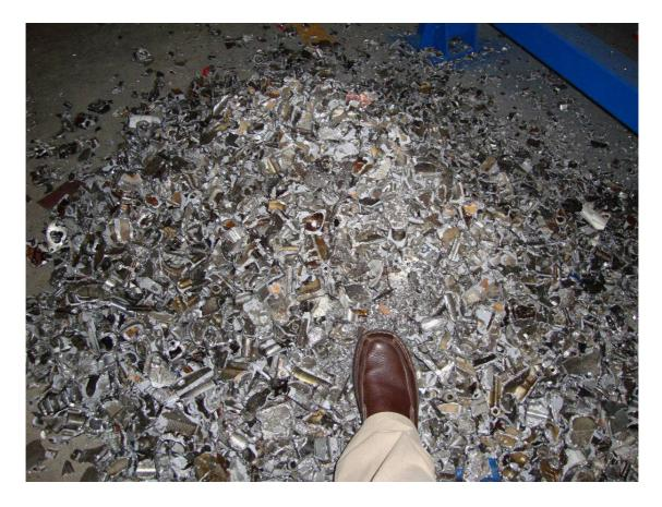
THIS IS AN EXAMPLE OF THE SECONDARY SHRED MATERIAL AFTER FERROUS REMOVAL
