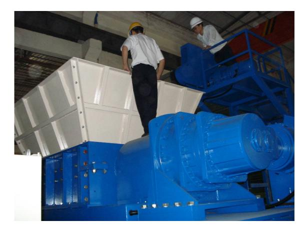
TO SHRED METAL IN A SHEAR SHREDDER ON A SUSTAINED BASIS YOU MUST HAVE A VERY LARGE AND VERY POWERFUL SHEARING TYPE SHREDDER TO CUT THE SCRAP METAL INTO STRIPS SO THAT IT CAN BE DENSIFIED INTO A FRAG.
