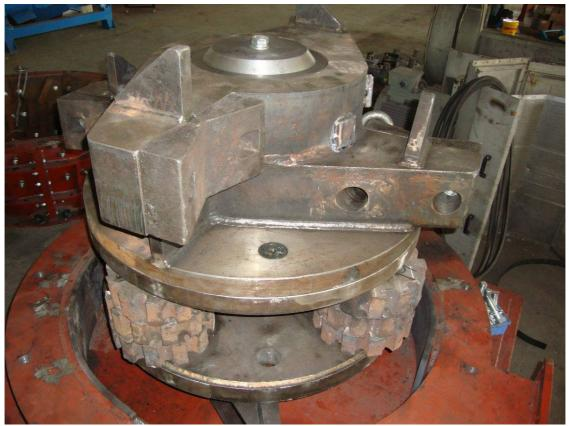
THIS SHOWS THE TYPICAL ROTOR DESIGN FOR DENSIFICATION OF SCRAP METAL AFTER IS IT CUT BY THE SHEAR SHREDDER PROCESSING LINE
