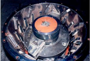
This is a top view of the Model V400 to densify the pre shredded scrap metal from the 7272 Shredder.
