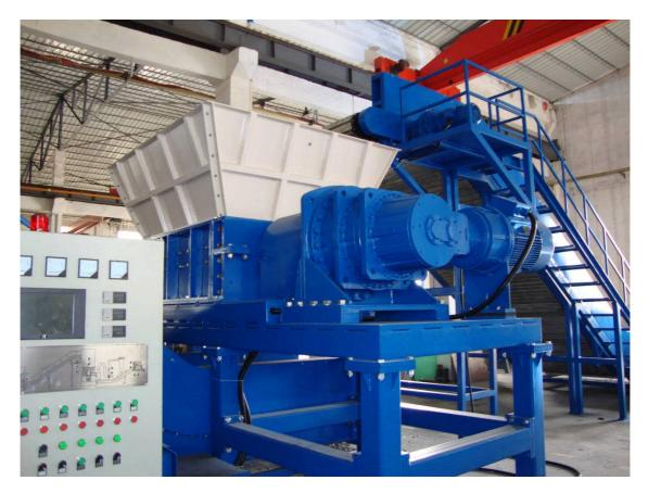
THE SYSTEM PROPOSED IN THIS DATA IS NOT DESIGNED TO SHRED WHOLE CARS WITH ENGINES AND AXELS. THIS SYSTEM IS DESIGNED TO SHRED WHOLE CARS WITHOUT ENGINED AND AXELS. HOWEVER IT CAN SHRED WHITE GOODS AND OTHER LIGHT STEEL, ELECTRONIC SCRAP AND OTHER SCRAP METAL THAT NEEDS DENSIFICATION OR SHREDDING.
