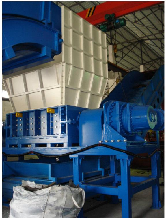
This is the primary shredder model 7272 shear shredder with a 24" shaft center distance to pre shred the car bodies.
