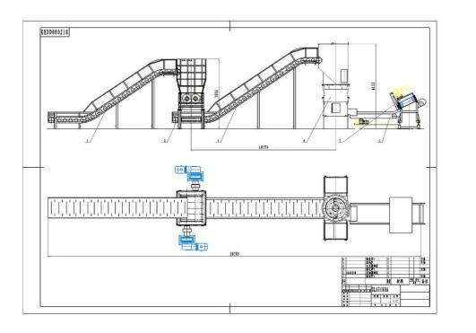
This shredding system uses two machines to take auto scrap to a frag form and the layout is shown in this drawing, and includes two steel belt conveyors for infeed of the primary shredder and infeed of the secondary vertical ring grinder-hammermill, and a single discharge conveyor and magnetic ferrous removal system, all offered for a system price of \$750,000.00.
