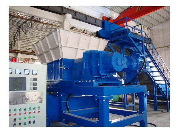
OVERALL THE BASE SCRAP METAL SYSTEM REVOLVES AROUND THE BASIC DESIGN THAT USES ONE OR TWO SHEAR SHREDDERS, AND ONE VERTICAL DENSIFIER.
