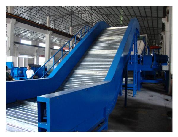
This is a picture of infeed and discharge conveyors that are used in the system. Although there are three conveyors in the picture the system uses two of these conveyors for the infeed of material into the primary shredder and for the discharge and infeed of material into the secondary shredder.
