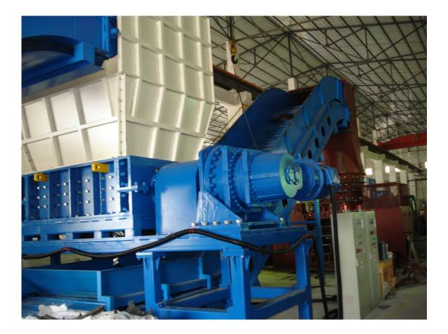
BASIC 7272 UNIT FOR SCRAP METAL PROCESSING OR FOR TIRE PROCESSING OR FOR MSW OR BULKY WASTE PROCESSING.
