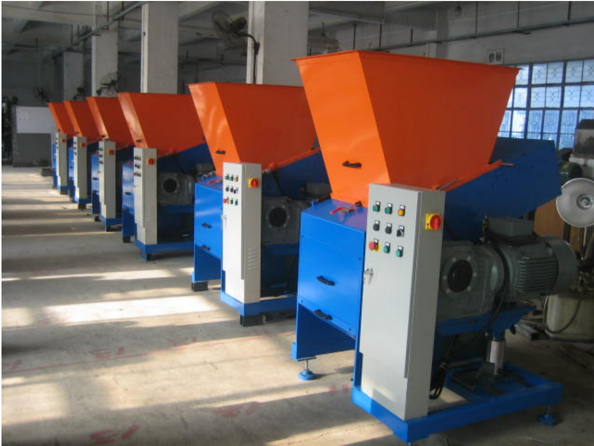
This is a picture of multiple 2024 A units with a 15 Hp drive. The same unit can be provided with a 20 Hp drive.
