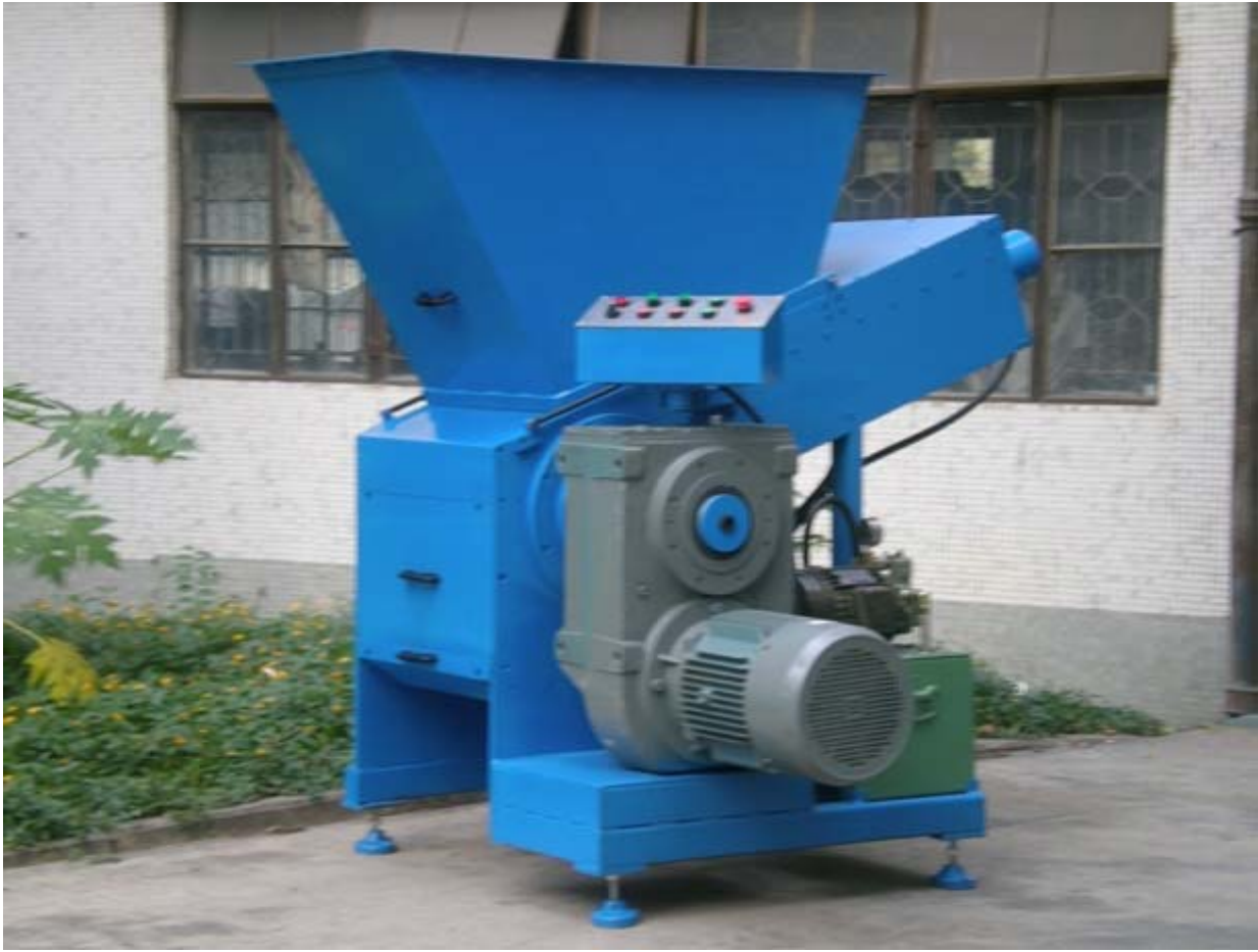
One Global Development Model 2024V-A Single Shaft Grinder with a 15 Hp drive.
