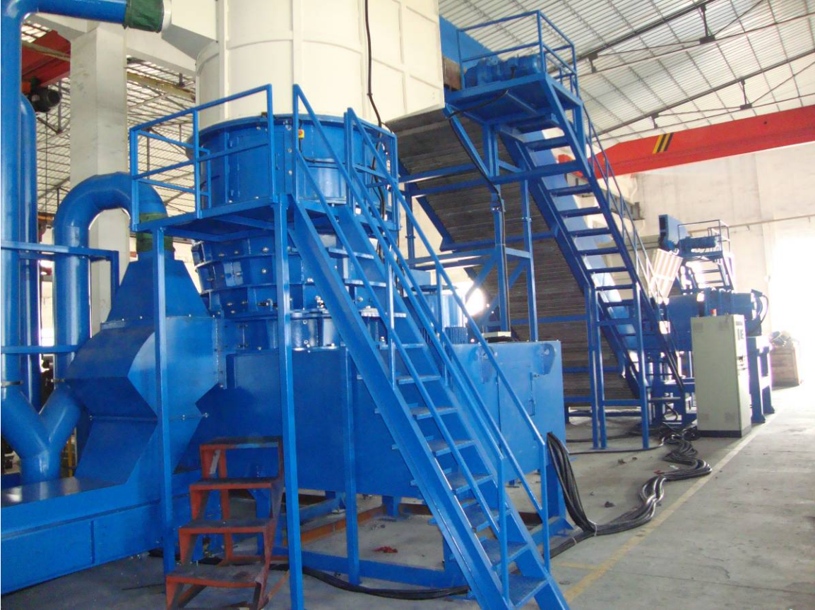
This is another view of the two meter wide secondary infeed conveyor that takes the primary shredded material into the vertical grinder.
