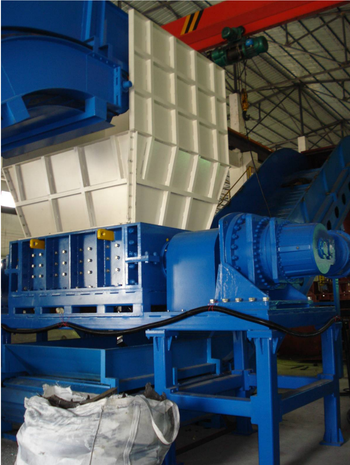
This is the primary shredder model 7272 shear shredder with a 24" shaft center distance to pre shred the car bodies.
