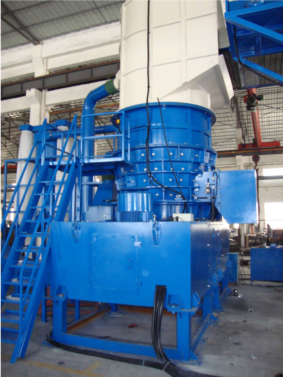
This is a picture of the Eidal V400 Grinder with infeed hood.
